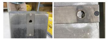
Example of a shutter fully open (left) and a shutter that is half-open (right) The best practice to confirm that a shutter is closed is to use a survey meter, however, there are other methods. The use of a mirror is one method which minimizes unnecessary radiation exposure to the worker.
