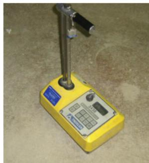
Two types of radiation are used in gauges: gamma (such as cesium-137) and neutron (such as americium-241/beryllium).
