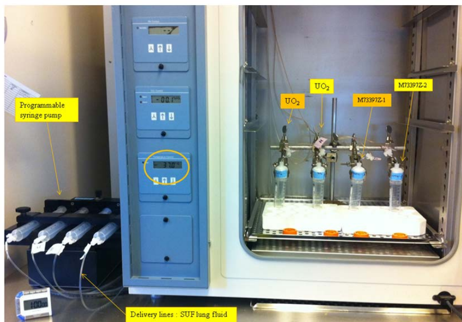
Figure 31 Experimental set up for the flow test. Flow rate: 0.46 \mu\text{L}/\text{min} ; Temperature: 37 \pm 0.5 \text{ }^\circ\text{C} ; pH: 7.4 \pm 0.2 ; Time points 24, 48, 72, 168, 336, 504 and 720 h.
