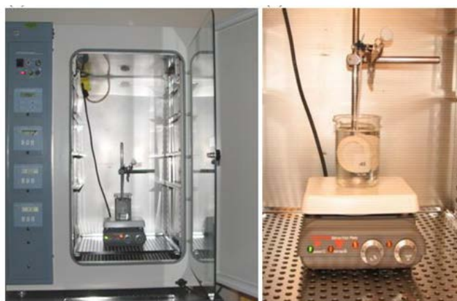
Figure 25 Static test set-up within an incubator for a controlled environment.
