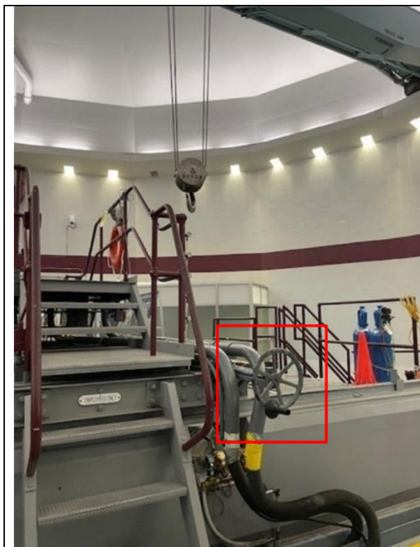
Figure 3. Photo to show the wheel that is used to move the reactor bridge. The yellow crane slings got caught on the wheel while the crane was moving upwards.
