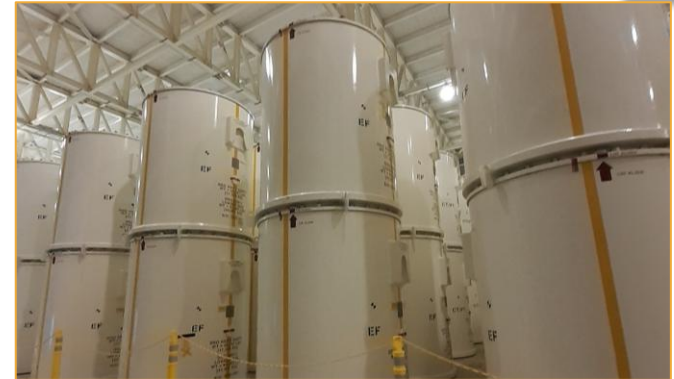
Darlington Storage Overpacks for ILW from refurbishment located at the Darlington Waste Management Facility
