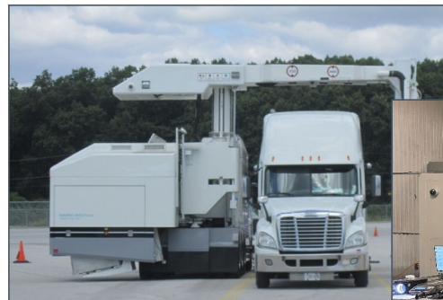
A linear accelerator that scans transport truck cargo
