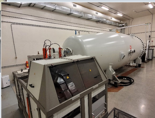
A tandetron, a type of high voltage particle accelerator
