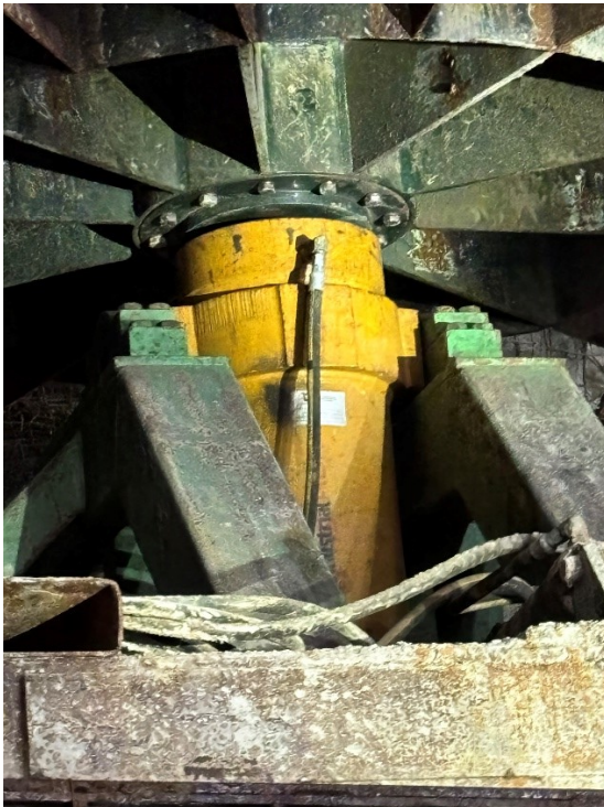
Figure 3: Close-up view of the bolts located on the flange of the 'pizza pan' above the hydraulic cylinder (Source SK LRWS)
