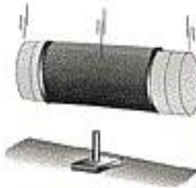
Drop from 1 m on a punch bar
