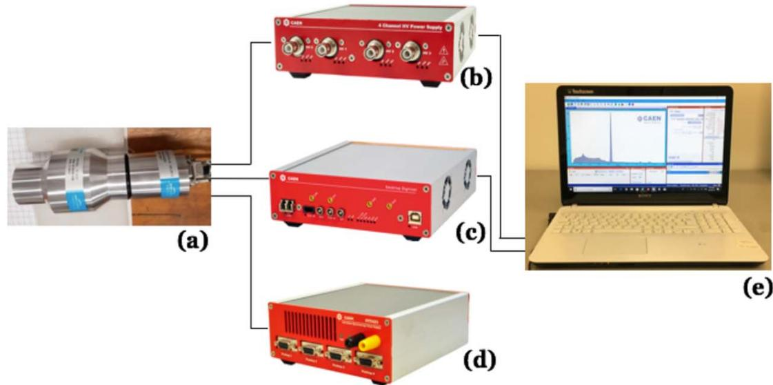
*Gamma spectroscopy system consisting of (a) LaBr<sub>3</sub>(Ce) detector, (b) HV power supply, (c) Digital pulse processor, (d) Preamp power supply, and (e) Data collection laptop*
