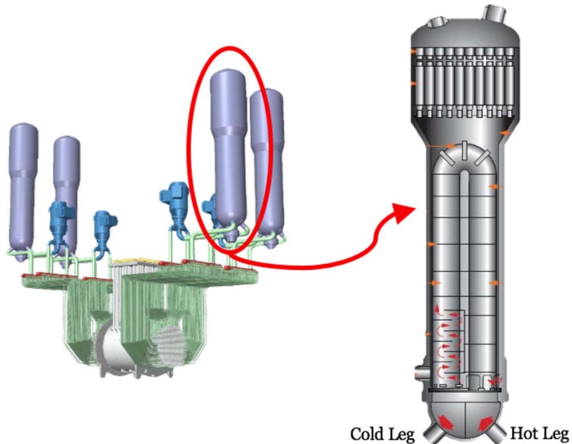
CANDU reactor (left) consisting of calandria, feeder pipes, headers, etc., with a zoomed in boiler (right), showing the hot and cold leg, where PHT water from core goes in and out, respectively.
