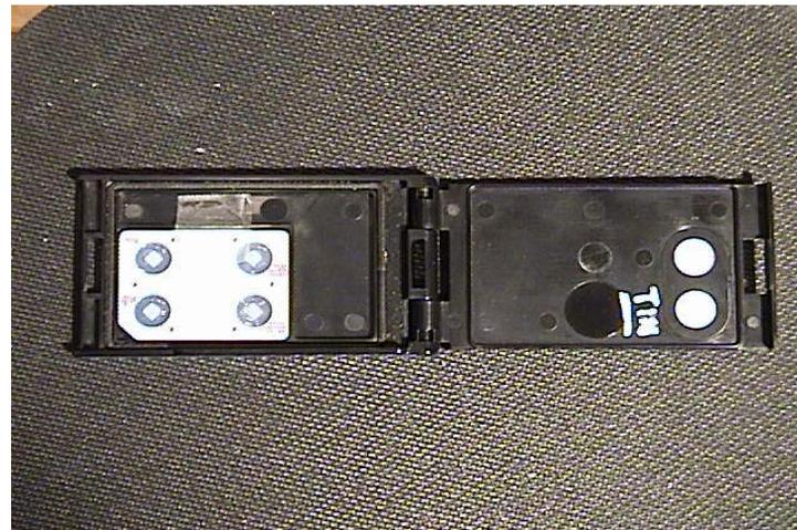
OPG 4 element dosimeter capable of measuring  $H_p(10)$ ,  $H_p(0.07)$  and beta/gamma components of  $H_p(0.07)$ ,
