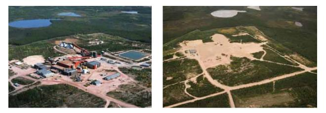
**Figures 7.2 (a) and (b)** – (a) A photograph of the mill areas during operation, and (b) a photograph of the area following decommissioning but prior to the re-vegetation becoming established.
