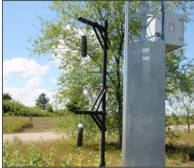
Figure 4: Passive sampler for tritium in air at a tritium-processing facility [28]
