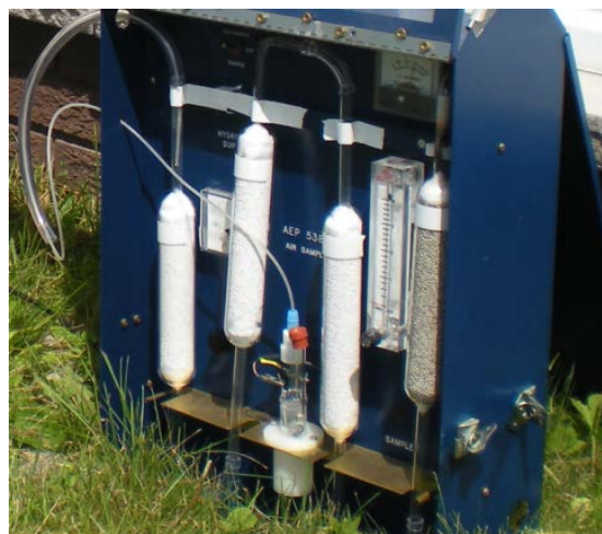
Figure 5: A Canadian Nuclear Laboratories (formerly Atomic Energy of Canada Limited) active sampler for tritium in air using molecular sieves [29]
