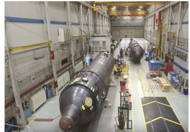
Steam Generators being assembled in BWXT's nuclear clean room in Cambridge, Ontario
