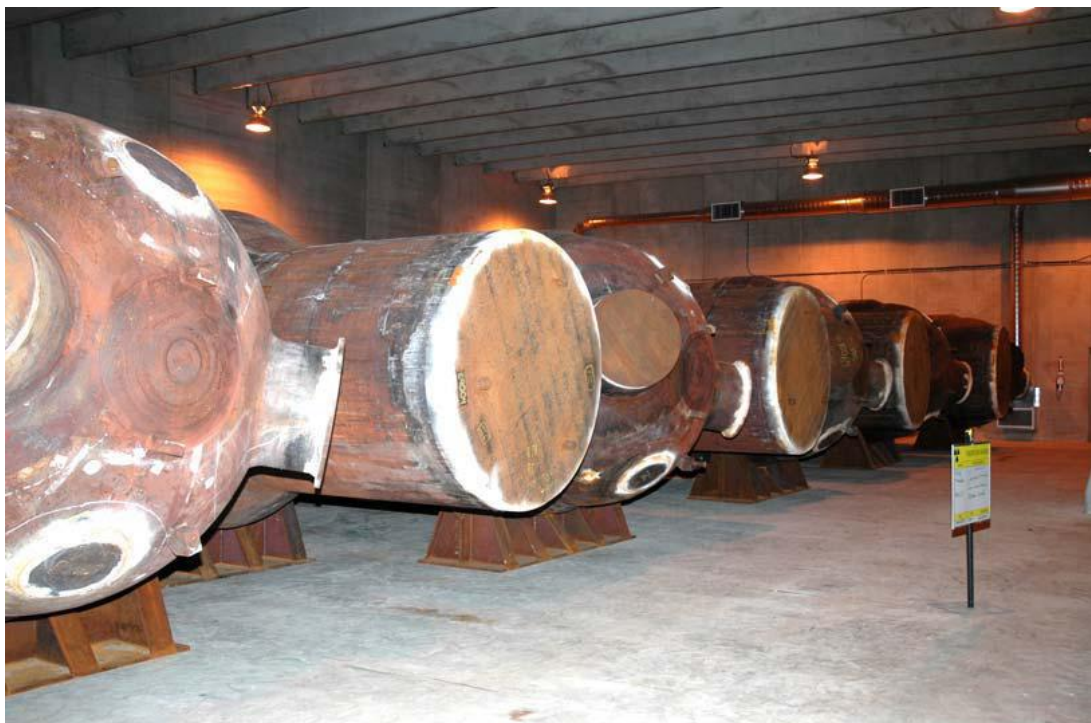
Figure 12: Storage of Steam Generators
