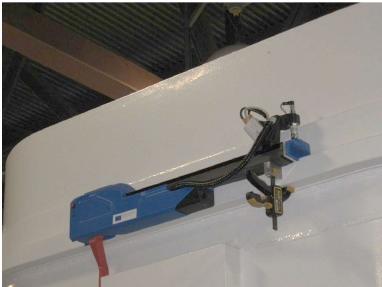
Figure 35: Laser Mapping Container Verification (LMCV)
