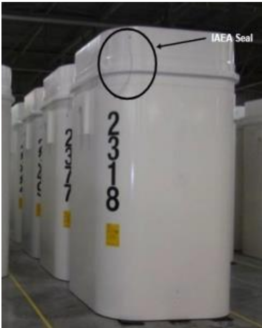
Figure 41. DSC in Storage showing IAEA Cobra Seals
