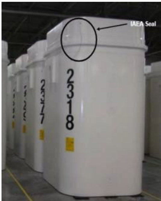
Figure 33. DSC in Storage showing IAEA Cobra Seals
