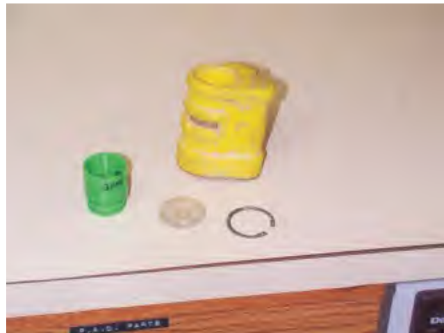
FIG 9 - Personal alpha dosimeter (PAD) worn on underground workers' belts. This device samples the mine air to determine monthly exposure to radon progeny and long-lived radioactive dust.
