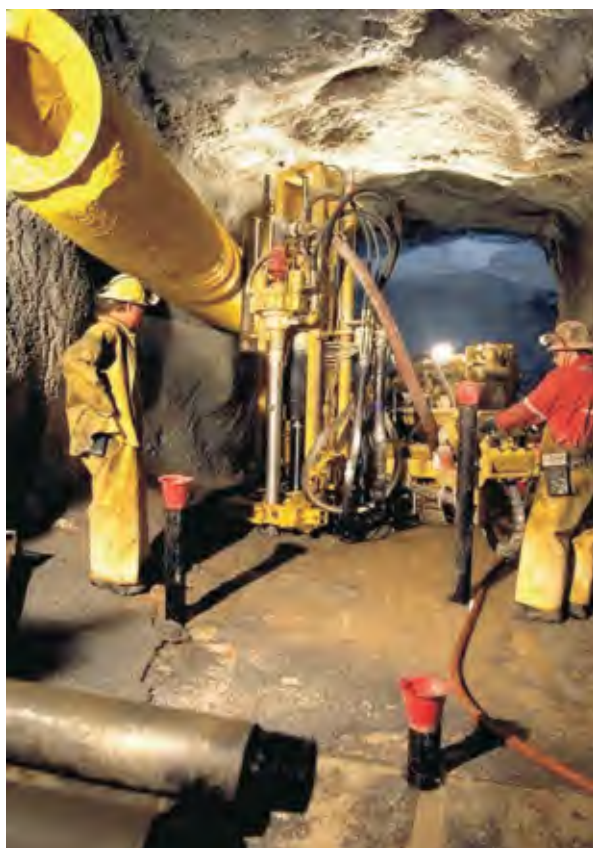
FIG 8 - Reverse circulation in-the-hole hammer blasthole drilling at Eagle Point mine. Note floor concrete and wall shotcrete for gamma radiation shielding from the orebody.
