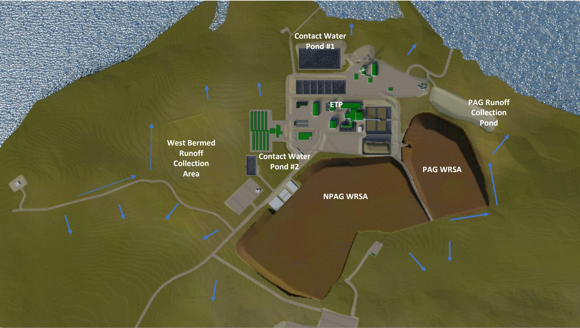
Figure 2: Surface Water Management: Non-Contact Water Diversion (Simplified Diagram)
