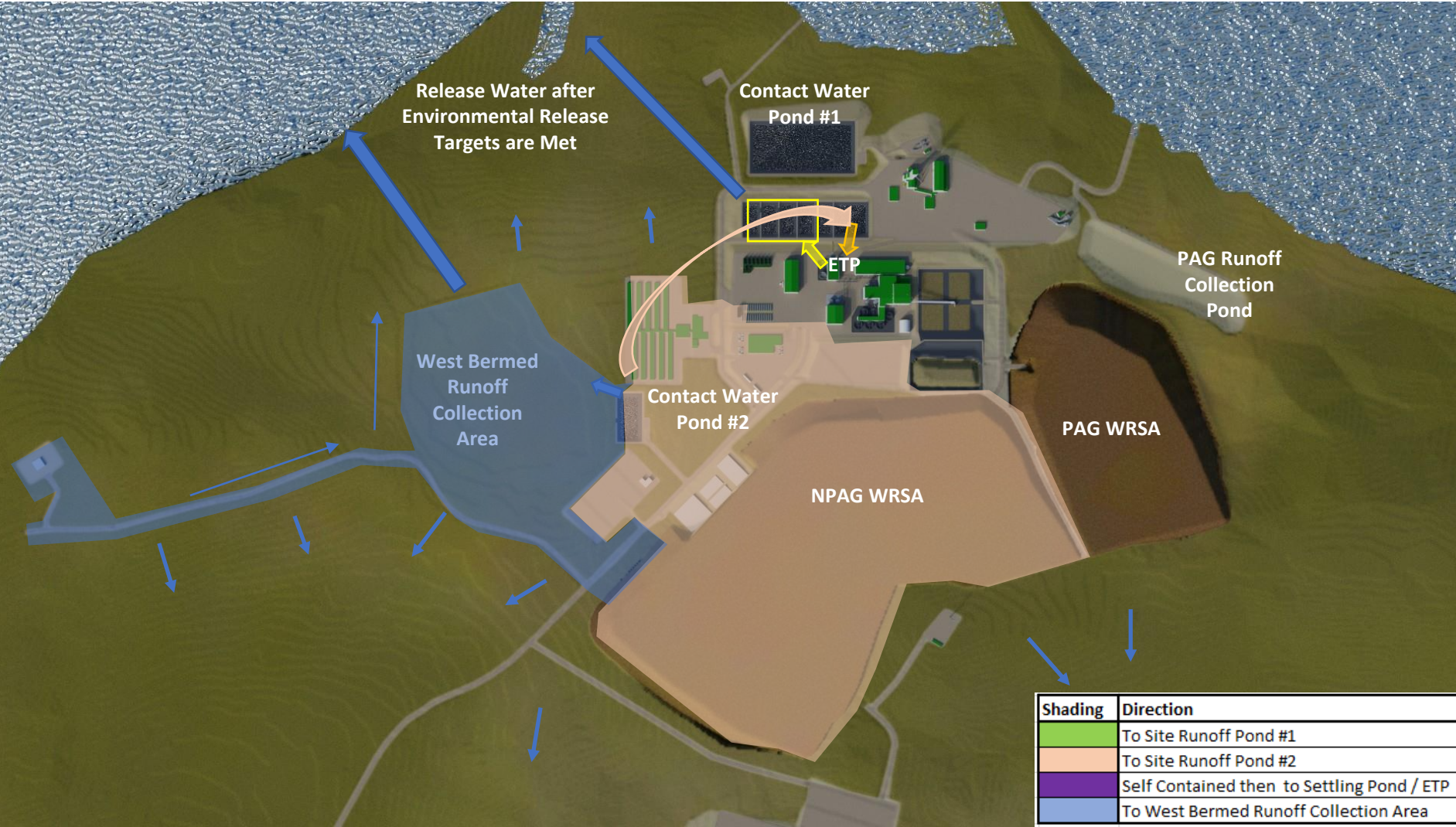
Figure 5: Surface Water Management: Contact Water Pond #2 / West Bermed Runoff Collection Area Drainage (Simplified Diagram)
