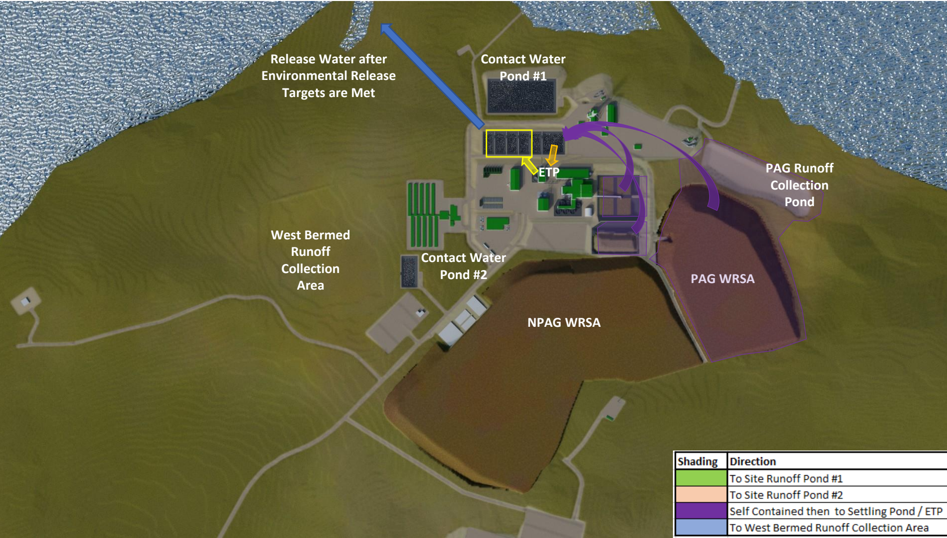
Figure 3: Surface Water Management: Self-Contained Contact Water (Simplified Diagram)
