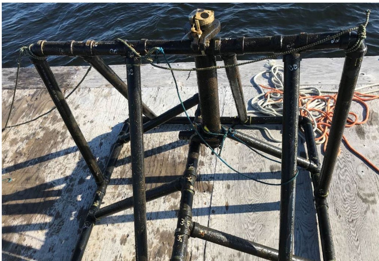
Figure 5: Nortek Aquadopp Acoustic Doppler Current Profiler and Mounting Frame Deployed at Patterson Lake North Intake
