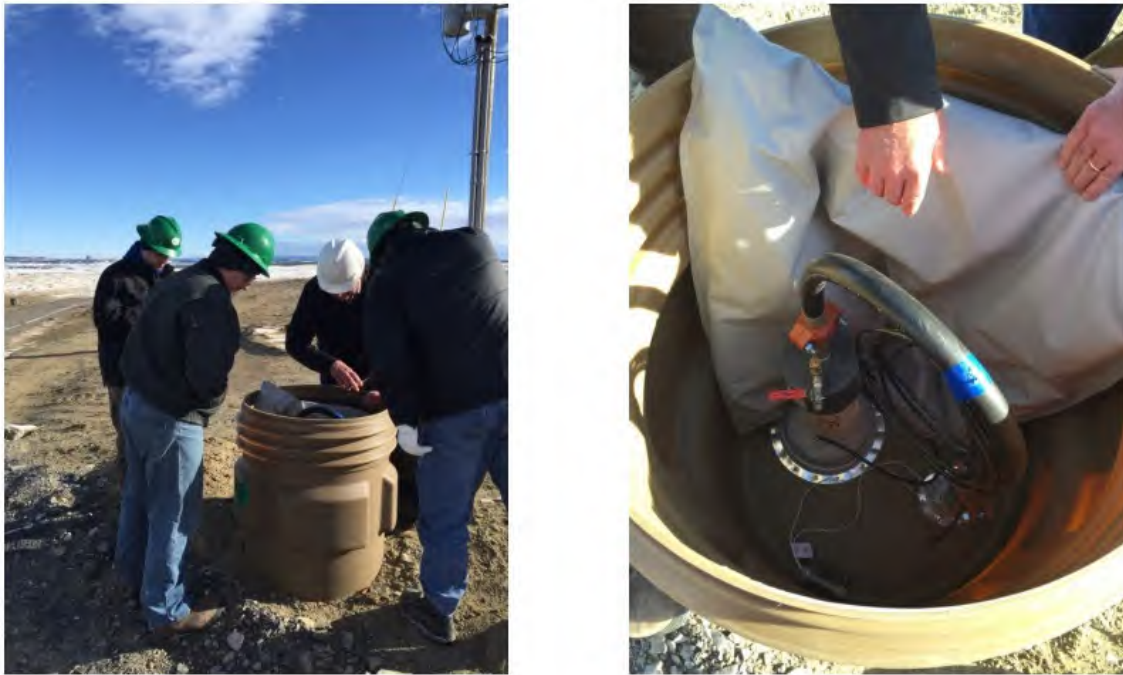
Figure 2.2-9: Typical In Situ Recovery Well at Surface
