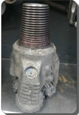
Mud rotary drilling bit
