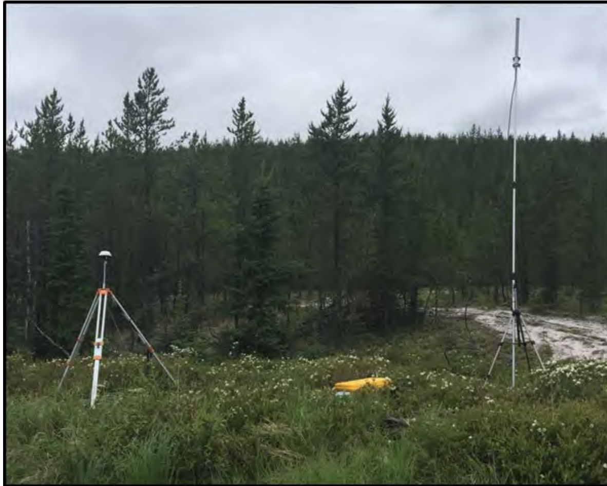
Figure 3. Shown is the Real-time Kinematic (RTK) GPS base-station and radio modem set-up on Lake LA6. A similar setup was deployed at Lake LA1.
