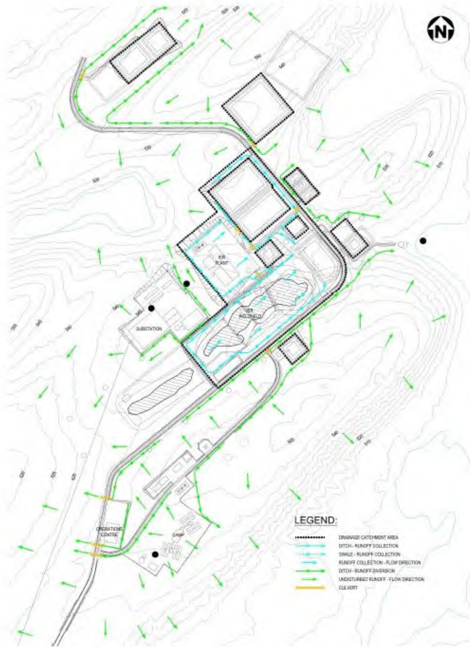
Figure 2.2-17: Site Drainage Plan with Flow Direction and Culvert Locations
