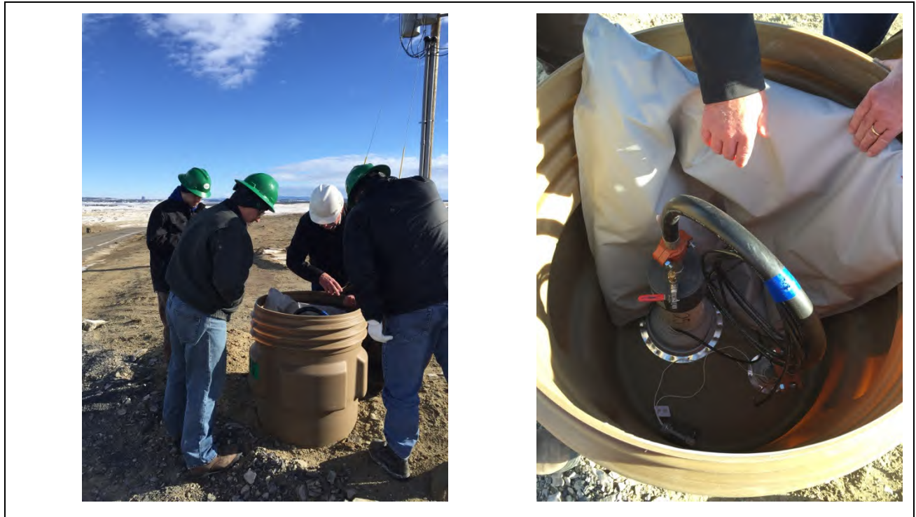
Figure 2.8: Typical In Situ Recovery Well at Surface
