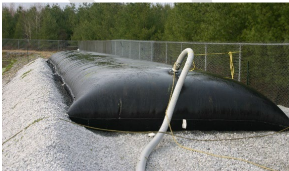
Figure 7: Example Geotube Used for Effluent Precipitate Dewatering
