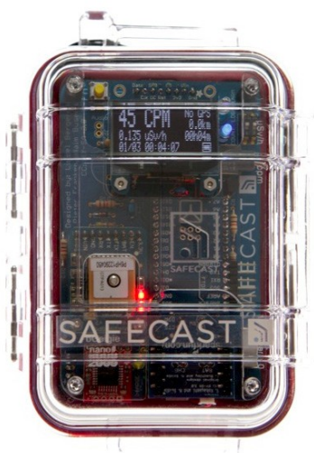
Figure 3: bGeigieNano portable radiation logging instrument.
