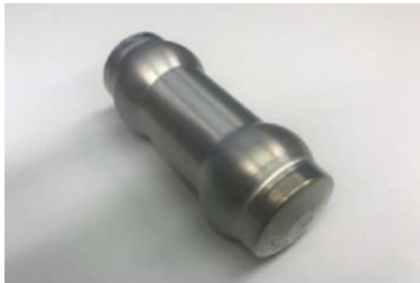
Figure 1. Exterior of Mo-99, ██████████, and Y-90 Target Capsule
