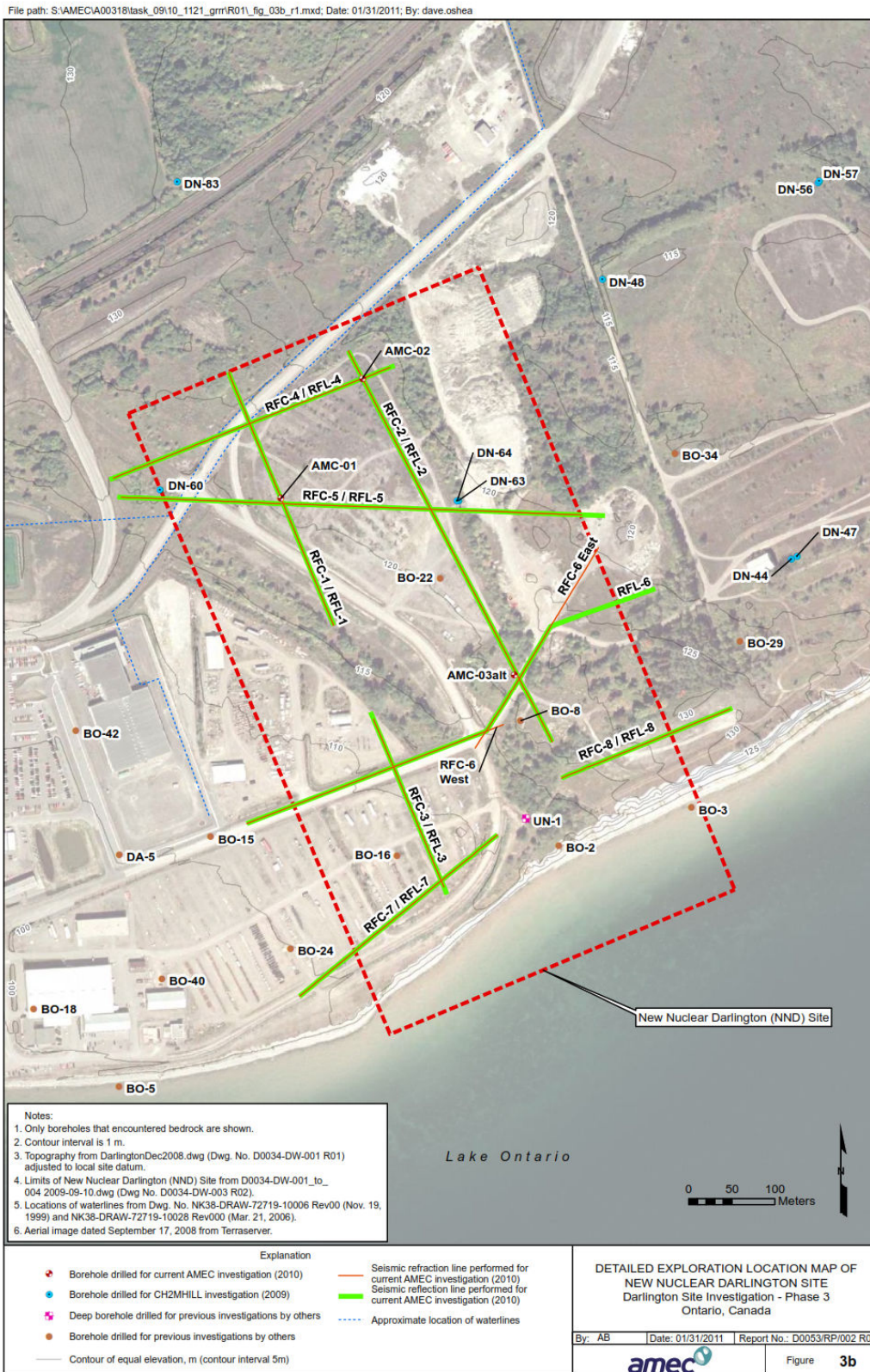
Figure 2.7.3.1-2: Locations of AMEC (2012) Boreholes (Reference 2.7-35)
