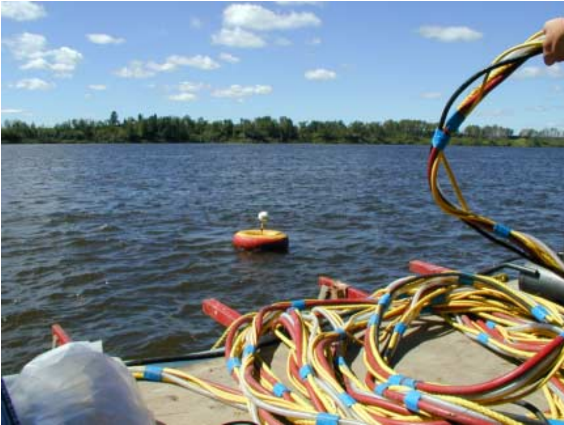
Figure 4 Use of GPS System to Log Underwater Survey Locations
