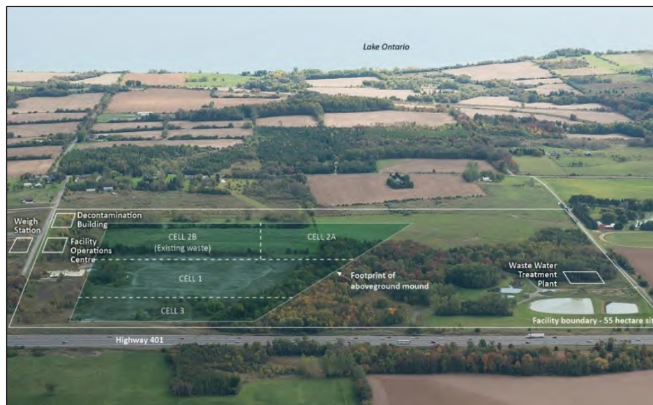
Figure 5: An overview of the site prior to Port Hope LTWMF construction, overlaid with LTWMF features (Source: CNL)
