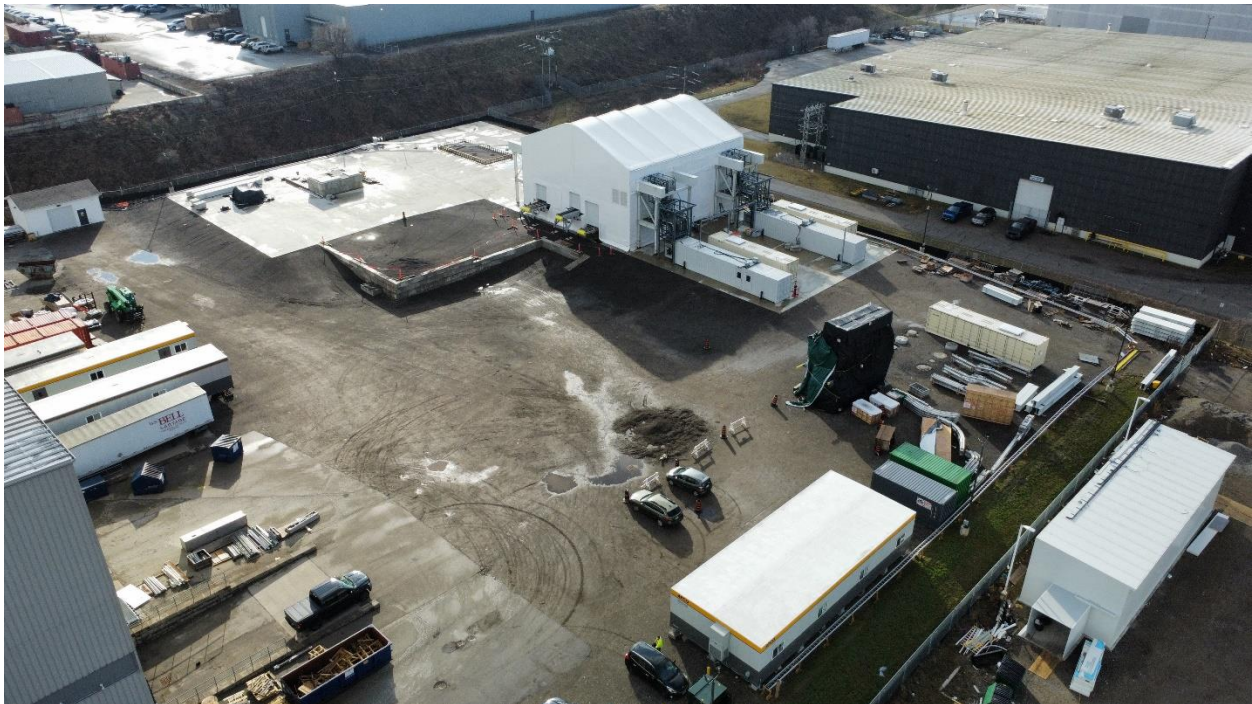
Figure 14: Aerial photograph showing the off site concrete pad that emulates site conditions with the waste retrieval system constructed on top for testing purposes.
