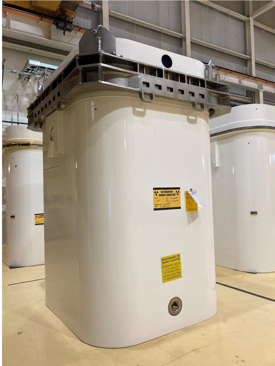
Figure A-3: DSC with Transfer Clamp Installed
