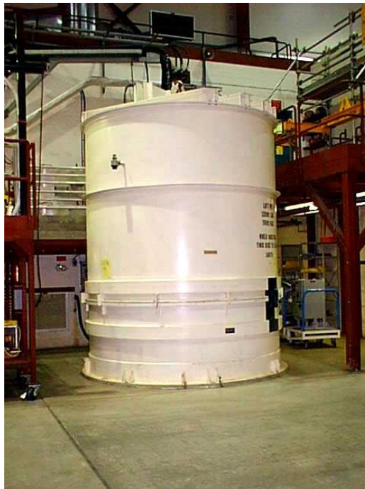
Figure A-14: The Dry Storage Container is Placed in the Helium Leak Test Vacuum Chamber under Vacuum and Inspected for Helium Leakage as a Final Test of the Seal Weld's Integrity
