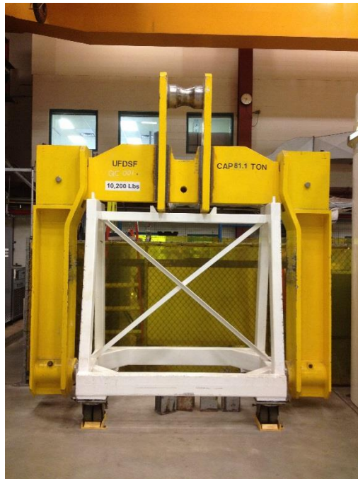
Figure A-6: The Dry Storage Container Handling System consists of Lifting Plates, a Lifting Beam, and a Lid Lifting Arrangement. The Lifting Beam is Visible in the Photographs
