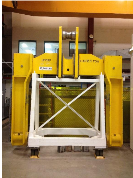
Figure A-8: The Dry Storage Container Handling System consists of Lifting Plates, a Lifting Beam, and a Lid Lifting Arrangement. The Lifting Beam is Visible in the Photographs
