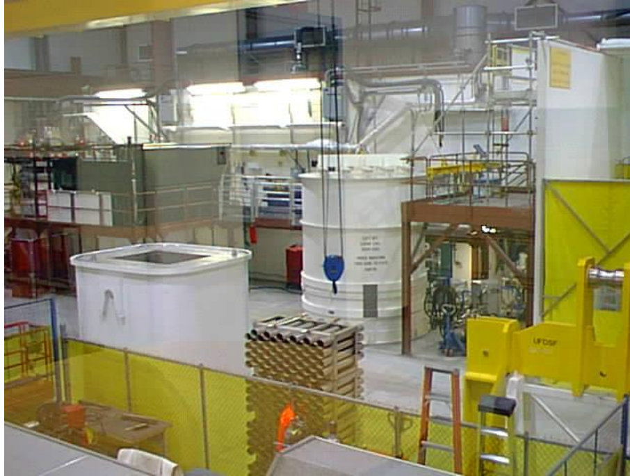
Figure A-7: Pickering Waste Management Facility Used Fuel Dry Storage Workshop showing an Empty Dry Storage Container Base, the Dry Storage Container Lifting Beam, the Overhead Crane, Welding Stations, and the Vacuum Chamber for the Helium Leak Detection System
