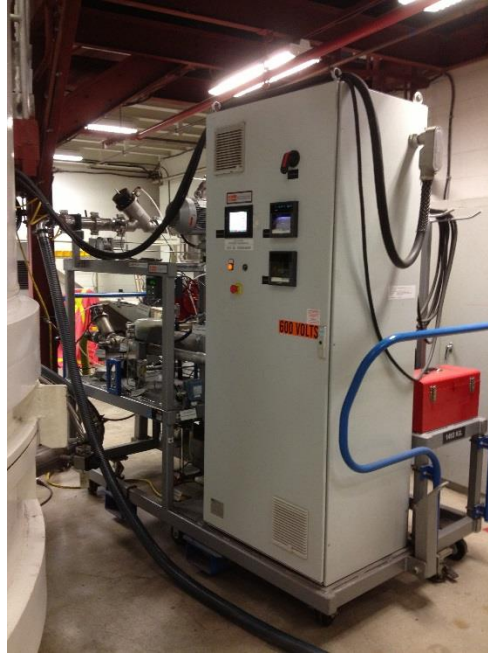
Figure A-10: Dry Storage Container Final Vacuum Drying and Helium Backfill Equipment
