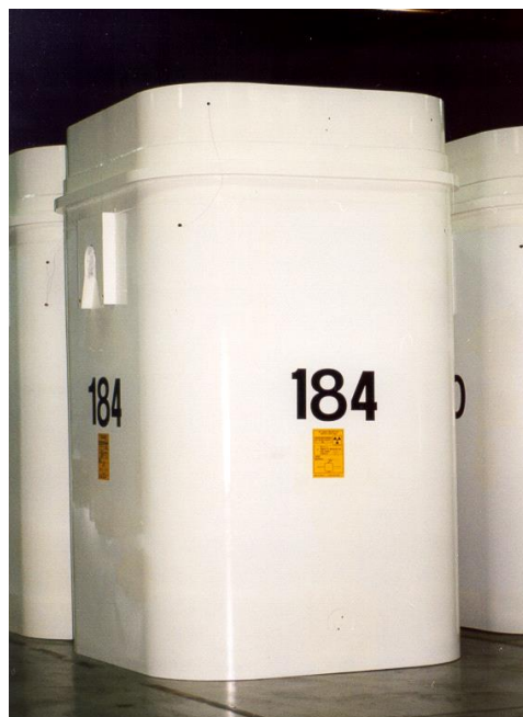
Figure A-17: Seal-Welded Dry Storage Containers in Storage
