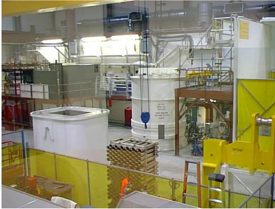
Figure A-5: Pickering Waste Management Facility Used Fuel Dry Storage Workshop showing an Empty Dry Storage Container Base, the Dry Storage Container Lifting Beam, the Overhead Crane, Welding Stations, and the Vacuum Chamber for the Helium Leak Detection System
