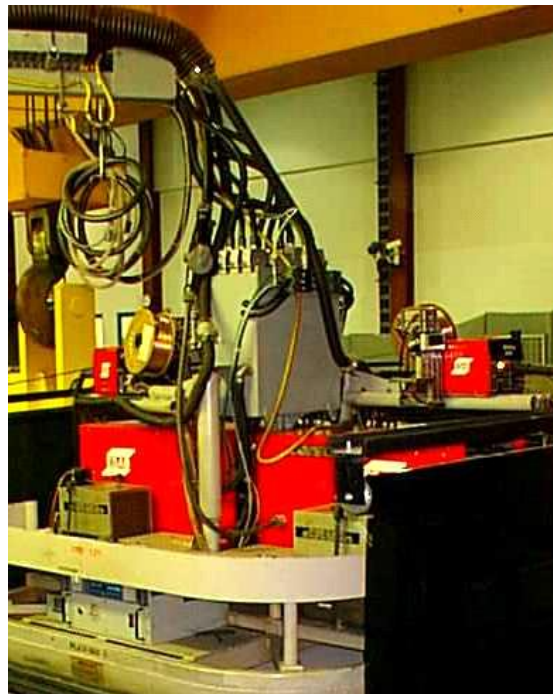
Figure A-10: An Automatic Dry Storage Container Lid Welding Machine is Used to Seal-Weld the Lid
