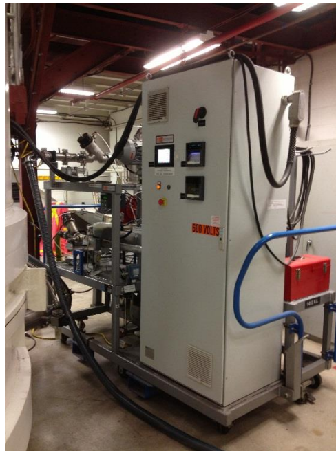
Figure A-8: Final Vacuum Drying of the Dry Storage Container Chamber is shown
