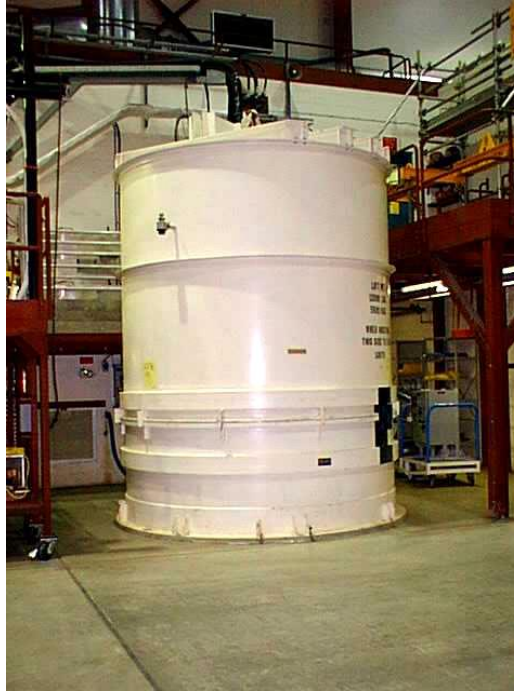
Figure A-16: The Dry Storage Container is Placed in the Helium Leak Test Vacuum Chamber under Vacuum and Inspected for Helium Leakage as a Final Test of the Seal-Weld's Integrity
