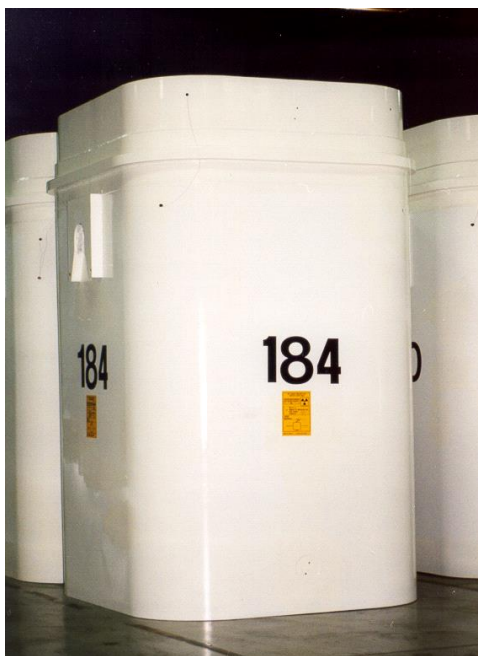
Figure A-15: Seal-Welded Dry Storage Containers in Storage
