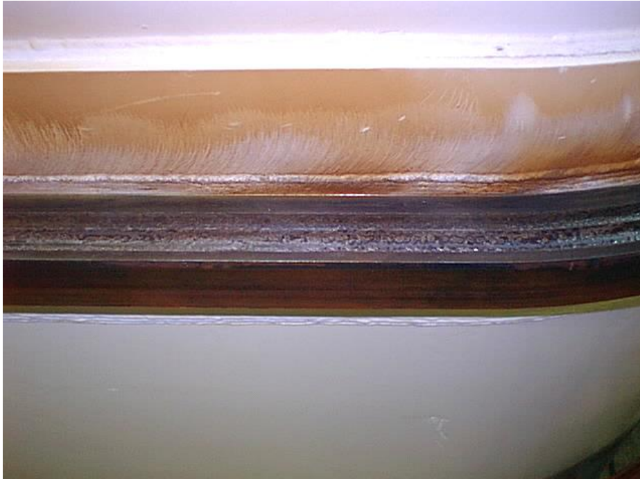
Figure A-11: Dry Storage Container Lid Weld – The Finished Weld is shown
