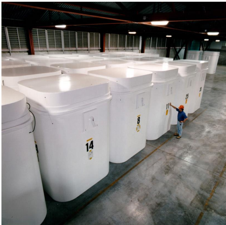
Figure A-16: Seal-Welded Dry Storage Containers in Storage
