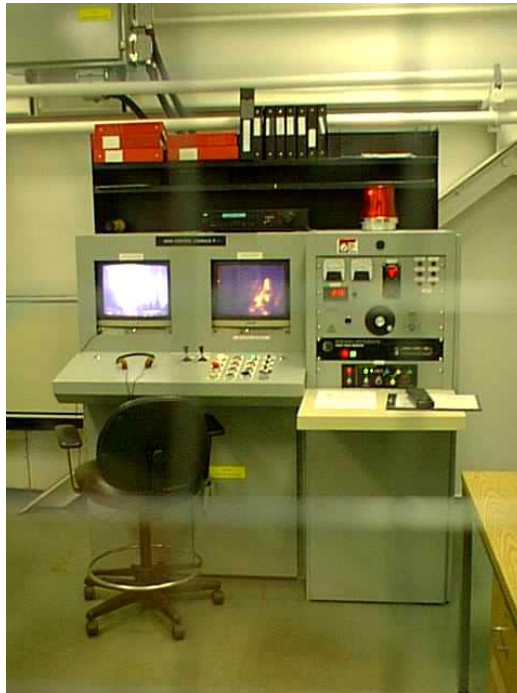
Figure A-9: Welding Control Room – The Welding Process is Monitored Remotely. The Screen shows the Weld Being Formed
