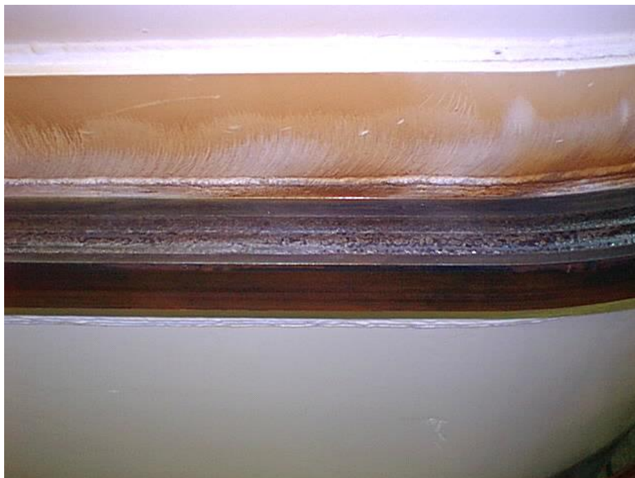
Figure A-13: Dry Storage Container Lid Weld – The Finished Full-Penetration Weld is shown
