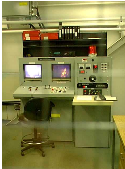
Figure A-11: Welding Control Room – The Welding Process is Monitored Remotely. The Screen shows the Weld Being Formed
