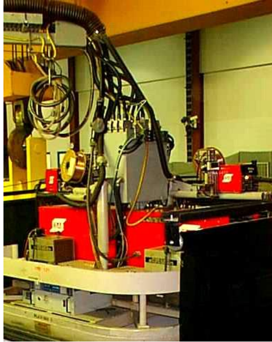
Figure A-12: An Automatic Dry Storage Container Lid Welding Machine is Used to Seal-Weld the Lid
