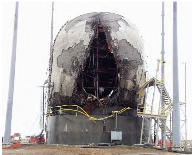
Figure 8 : Containments will not crack and reclose; they will burst. Results of SANDIA joint Japanese-U.S tests.
