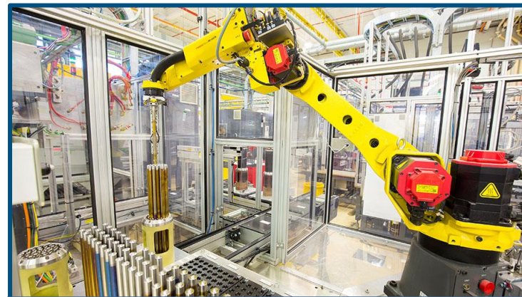
CFM robot inserting rods into fuel bundle assembly
