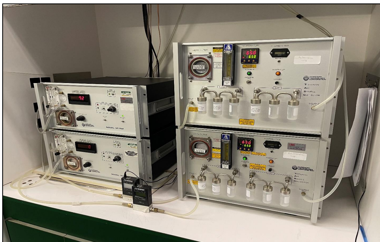
Figure 28: Equipment used to continuously monitor and measure gaseous releases of tritium through the active ventilation systems.
