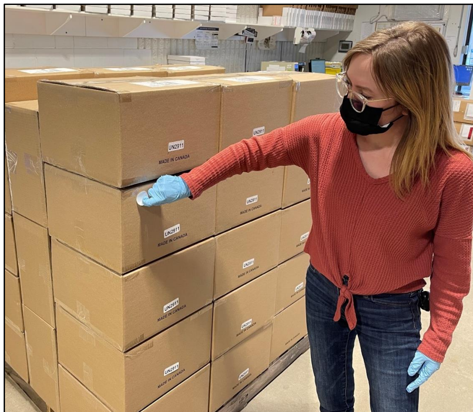
Figure 22: A member of the SRBT Health Physics Team conducts a removable contamination assessment of packages being readied for transport.
