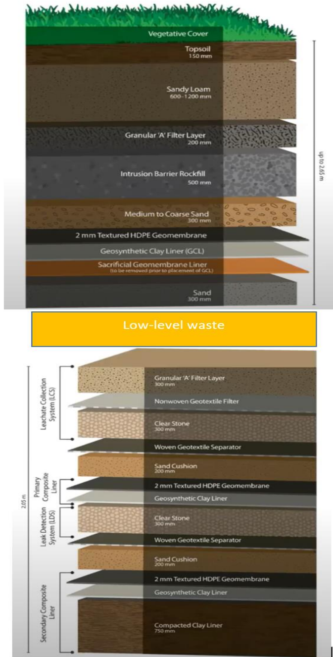
Figure 3 – NSDF ECM – Base Liner and Final Cover Systems (not to scale) Source: Adapted from CNL figures
