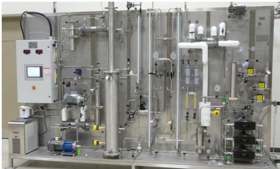
Figure 11 Performance testing wetproofed catalyst for hydrogen isotope separation processes, such as tritium removal and heavy water production.
