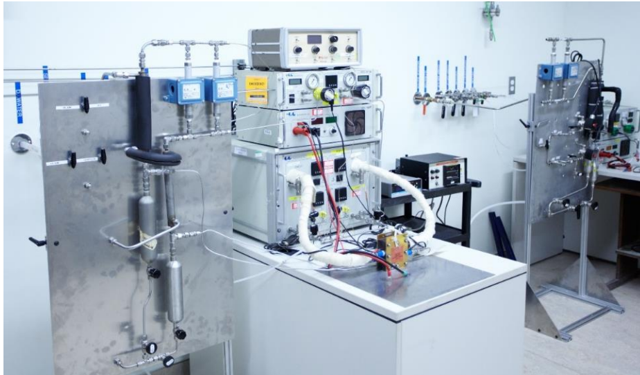
Figure 10 Testing hydrogen fuel cells to measure the performance of components developed at CNL, such as electrode catalysts and membrane materials.
