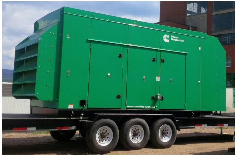
Figure 47 Mobile diesel generators (Fukushima Response Project).
