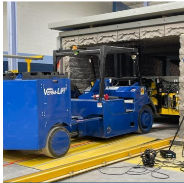
Prototype Remote Emplacement Equipment (courtesy NWMO)
