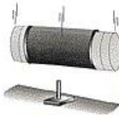
Drop from 1 m on a punch bar
