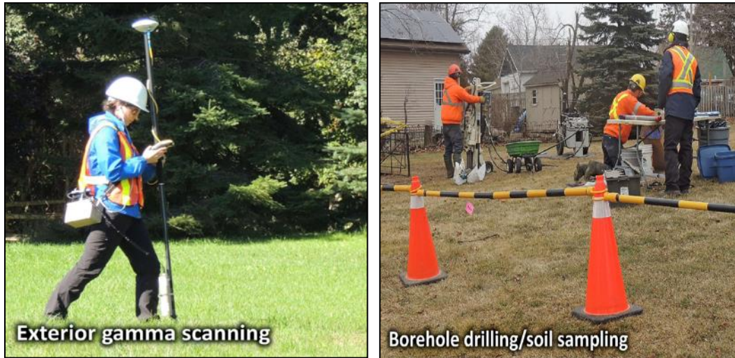
Figure 31: Exterior Gamma Scanning and Borehole Drilling/Soil Sampling
