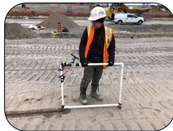
Performing an Electrical Leak Location Survey
