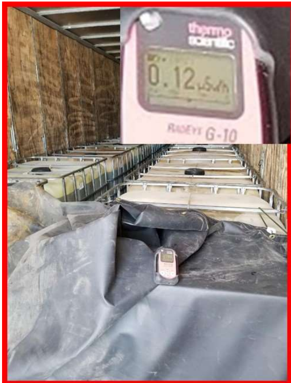
Interior of a container, with totes, and radiation survey meter showing a reading of 0.12 \mu\text{Sv/h} .
