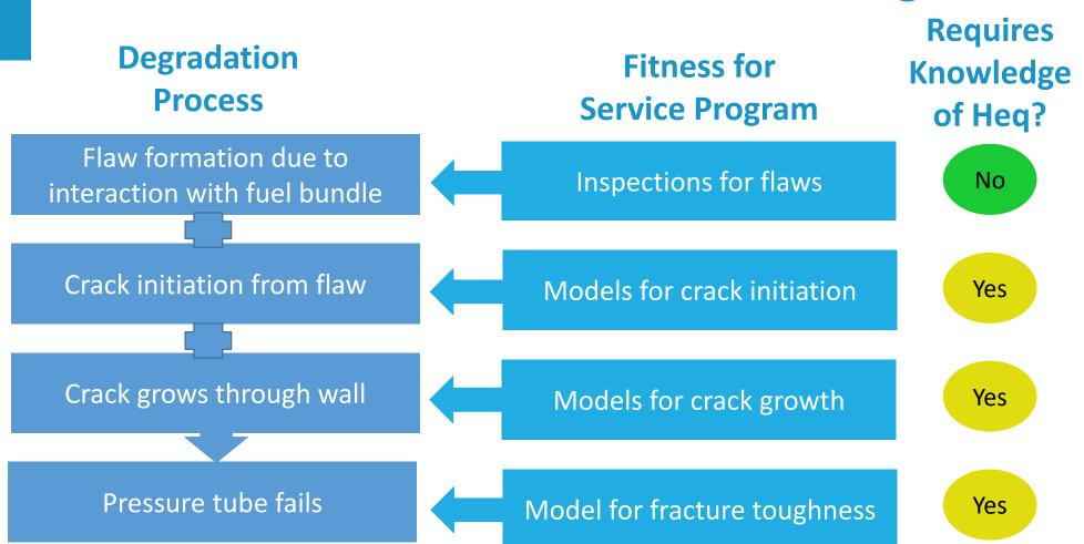
Presence of flaws in the region of interest is one of the conditions for pressure tubes crack initiation
