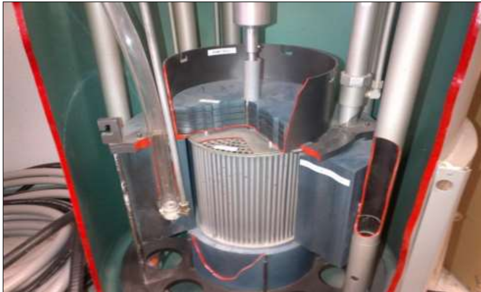
Figure 4-1: Model of a SLOWPOKE-2 reactor core (Source: RMC)
