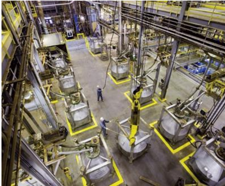
Blind River Refinery UO 3 tote bin loading area Source: Cameco
