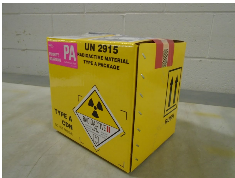
Figure 9: Example of Exterior of Typical Type A Transport Package
