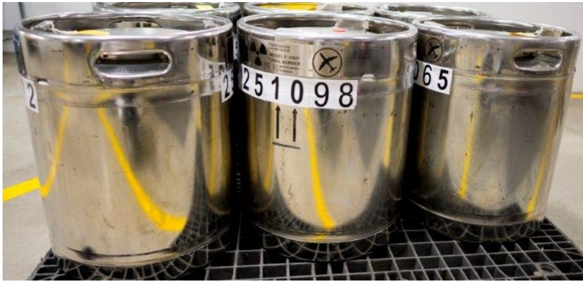
Figure 10: Example of Type B Transport Package
