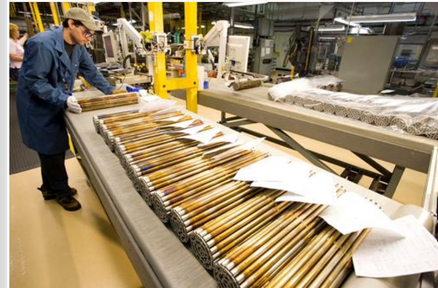
A CFM worker performing a final inspection on a fuel bundle prior to packaging.
