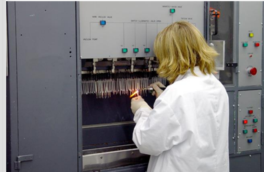
SRBT employee performing tritium filling operations Source: SRBT
