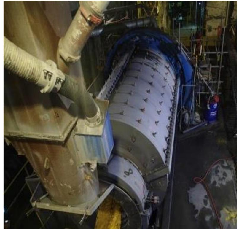
SAG mill used to grind ore at the McArthur River Operation.
