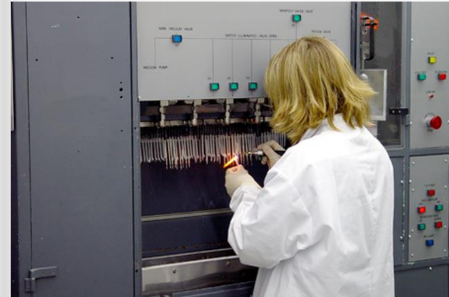
SRBT employee performing tritium filling operations Source: SRBT
