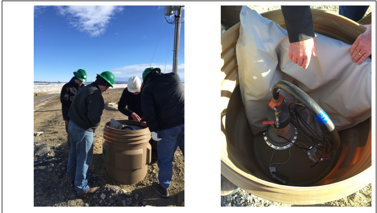
Figure 2.9: Typical In Situ Recovery Well at Surface
