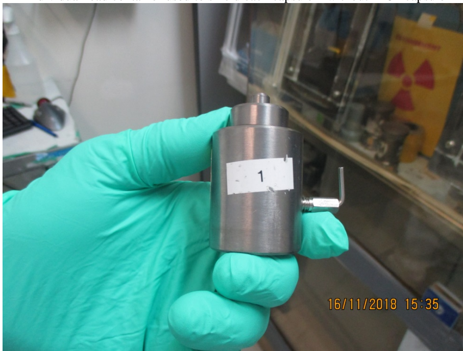
Individual lead container used to shield each capsule – without I-131 capsule
