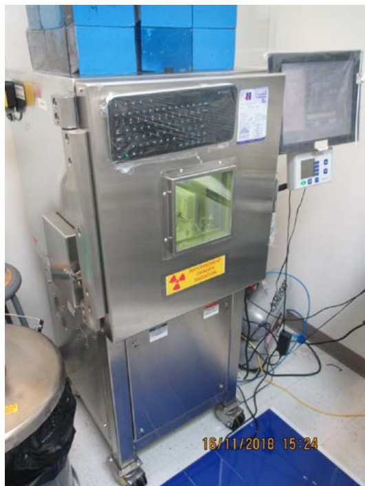
Picture 3. AseptiBot in use at Isologic for manufacturing the I-131 capsules
