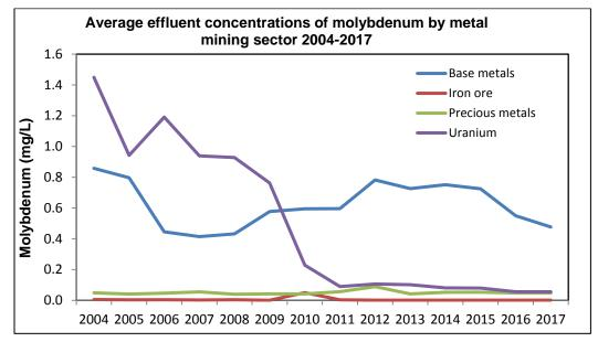
Figure 2.10: Average treated effluent concentration of molybdenum by metal mining sector, 2004–17
