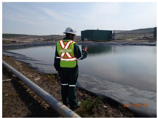
Figure 2.2: McArthur River - CNSC inspector measuring gamma dose rate
